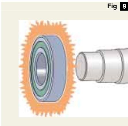
**Bearing on an SKF induction heater**
